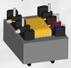
Other possible paths to consider are those between the primary winding turns and the secondary winding pins.
