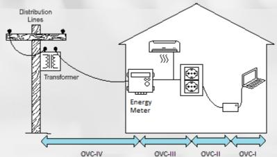
Depending on how the transformer is installed, it must comply with the adequate overvoltage category.
