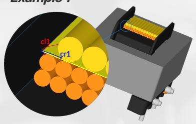
The drawing shows a transformer with primary winding (orange wire) and secondary winding (yellow wire) separated by yellow insulating tape, represented in cross-section.
