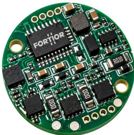
Figure: Joint drive for miniature robots using the FU7512Q
