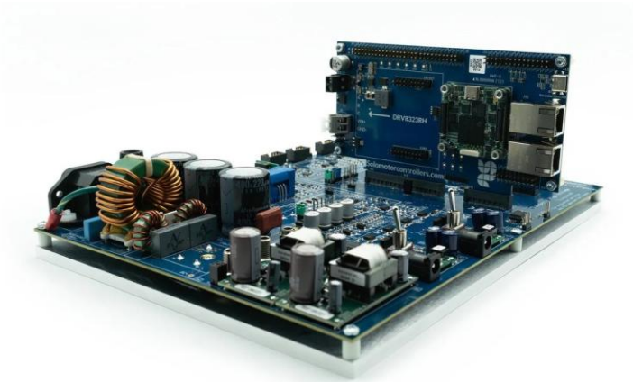
Figure 3: SOLO SOM Evaluation Board plugged into the 400 V development platform.
